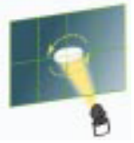
Contrast R + OMP (Prismatic glass with medium angle asymmetrical beam)
